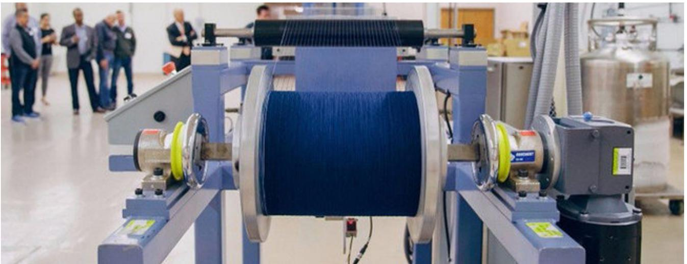
*The process involves the direct application of the mousse to the yarn - VF Corp*
